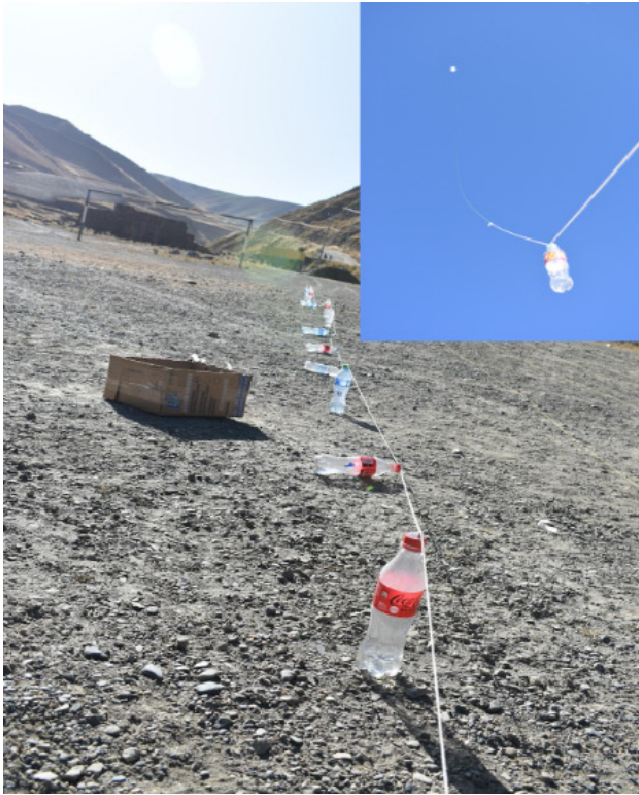
Fig. 2.— Manual tethered solution that required no power, permitted the balloon to fly freely on ascent thus permitting accurate wind measurements and was recoverable. The balloon at its highest ascent is shown in the upper right with the first water bottle lifted off the surface. The line of bottles ready to be lifted is shown in the main photo. Repeated profiles were successfully performed at all three experimental locations with these devices.
